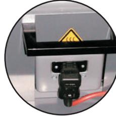
Latch / release the locking of the container
