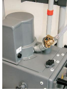
2.) assemble the control line of the refilling lance, plug it into the socket (**control line**) and lock it.
